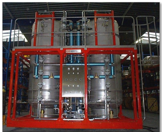
Hydrogen cryogenic purifier EF 450-250 450 Nm 3 /h - 250 Barg
