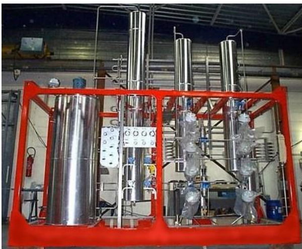
Hydrogen purifier D 900-250 900 Nm 3 /h - 250 Barg
