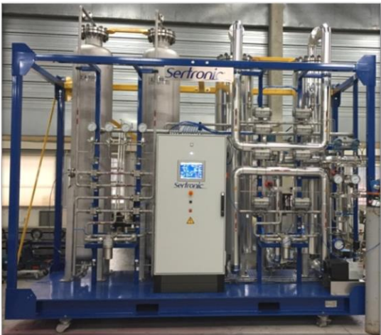
Helium dryer & CnHm removal 600 Nm 3 /h – 30 Barg
