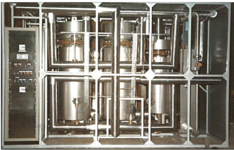
Oxygen purifier M 220-4 220 Nm 3 /h - 4 Barg
