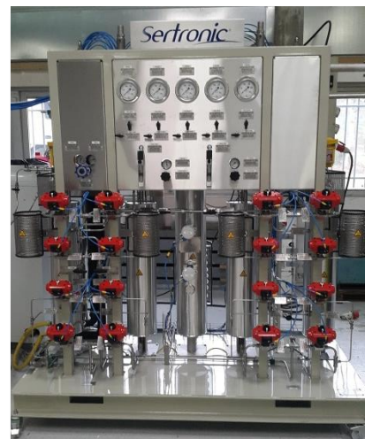
Hydrogen purifier D 16-165 16 Nm 3 /h - 165 Barg
