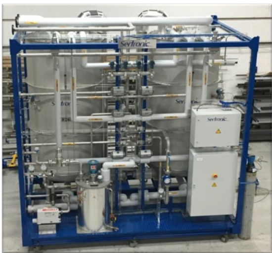
Helium cryogenic purifier EF 840-10 840 Nm 3 /h - 10 Barg
