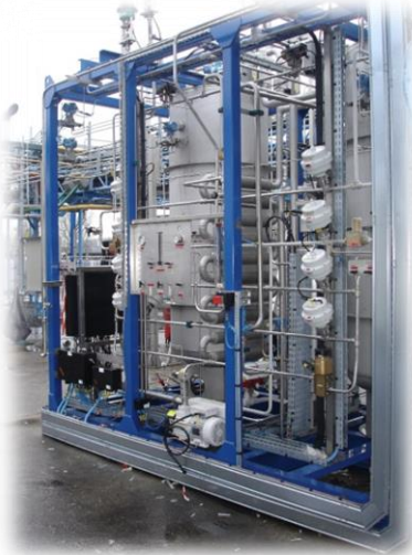
Cryogenic Hydrogen purifier 700 Nm 3 /h – 100 barg
